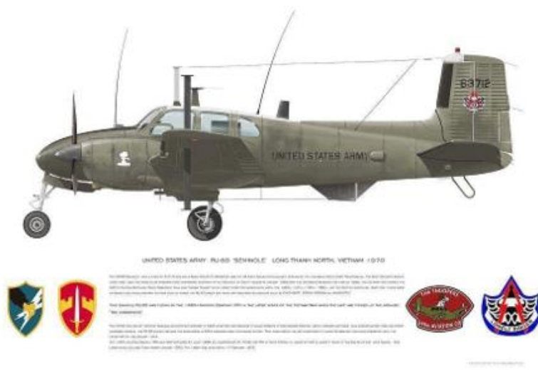
Beechcraft RU8D used for radio/voice intercept & aerial radio direction finding (ARDF) by triangulation of target.
